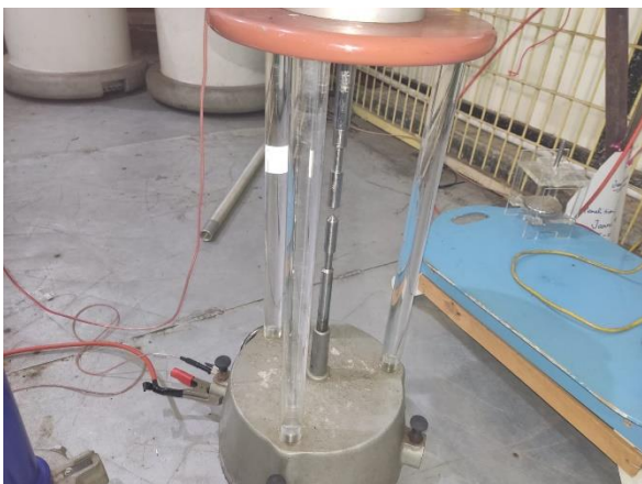
Measuring Spark Gap (MF)
